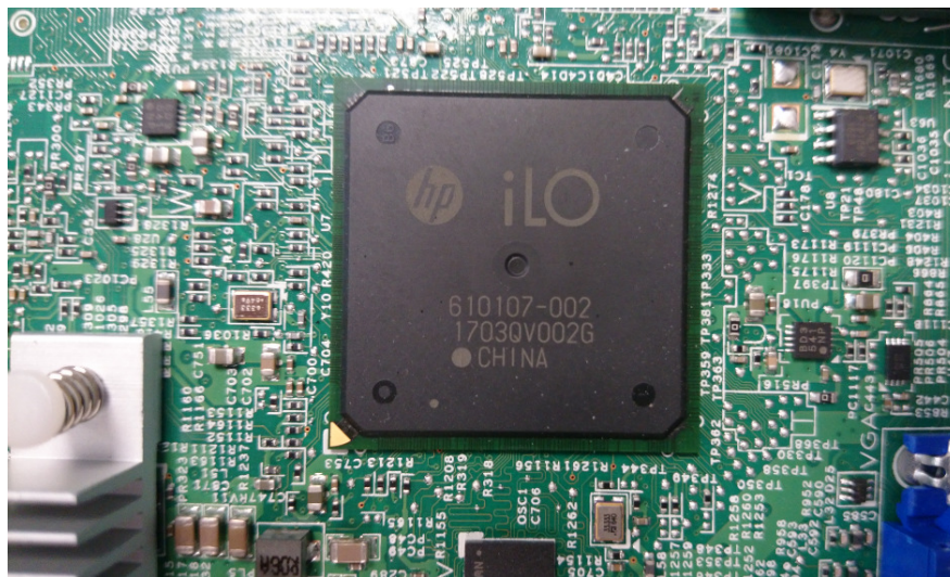
Fig. 1. iLO chip on server's motherboard
